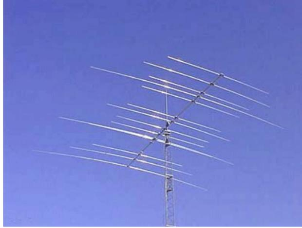
Figure 2: C-31XR 3-band Yagi Antenna
